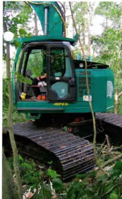
Powerful front tilting mechanism up to 15 degrees Tracks 1,300 mm wide
